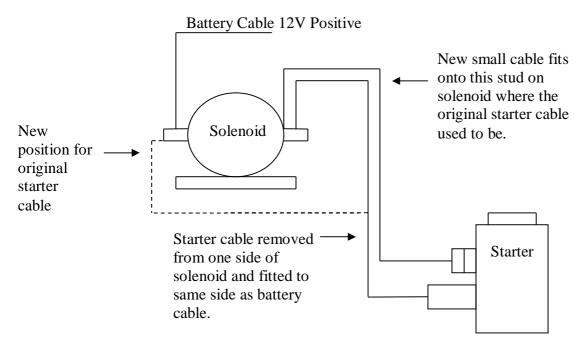
Two wires from the old lever starter switch, get joined to the two wires supplied with the Press Starter Switch.
